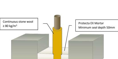
Protecta EX Mortar - Metal Pipe, Continuous Insulation in 100mm Concrete Floor
